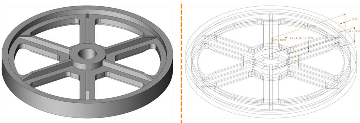
Figure 97 Case2 – Crank Pulley
