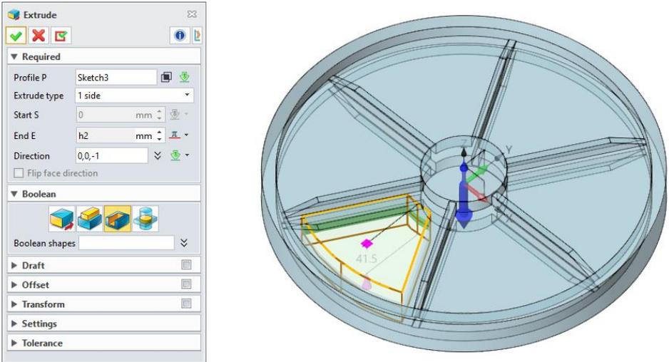
Figure 107 Case2 – Extrude Cut the Fan-shapes Hole
